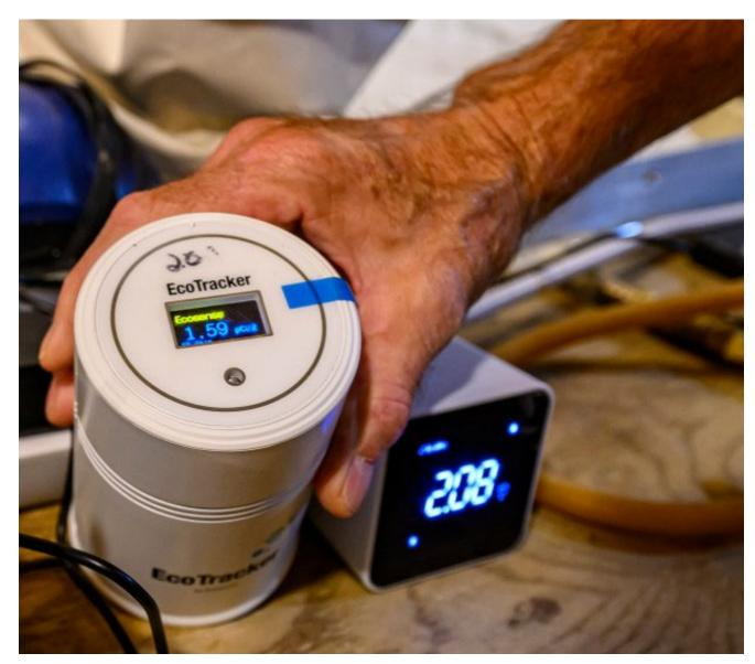
Bill Brodhead talks about devices used to detect radon including a radon chamber in his small radon lab in his basement Tuesday, April 18, 2023, in Riegelsville.
