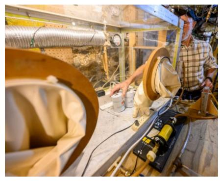
Bill Brodhead talks about devices used to detect radon including a radon chamber in his small radon lab in his basement Tuesday, April 18, 2023, in Riegelsville. Brodhead, one of the longestpracticing radon mitigators in the state, also teaches at Rutgers and has written papers and has done research on radon for the government. (April Gamiz/The Morning Call) Brian Yang first became aware of radon when his family moved from New Jersey to Center Valley two years ago.
